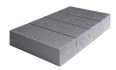
Unstressed insulation panel with increased density and low water absorption suitable for external thermal insulation systems of the perimeter areas of skirting, made of sintered expanded polystyrene (EPS) with the addition of graphite.
